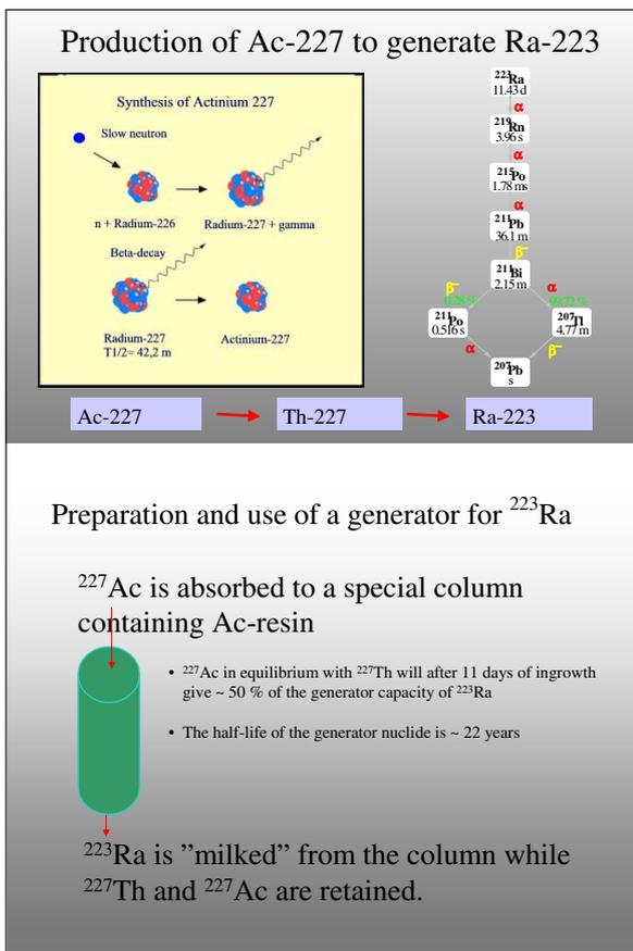
*Fig 1 A&B Production/Deacay scheme & Generator*
